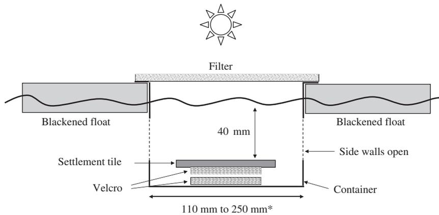
**Fig. 2** Experimental set-up. Cross-section of one experimental unit. The distance between water surface and settlement tile was 40 mm. \*, Length of unit depended upon latitude, and was such that the entire settlement tile was exposed to sun radiation for at least 2 h either side of noon.
